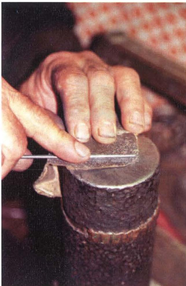
Fig. 7. Shaping the iron rod for the frame.
