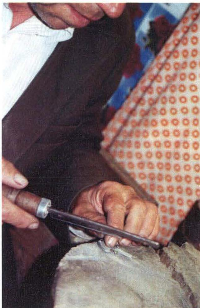
Fig. 11. Sawing the tongue's notch into the frame.
