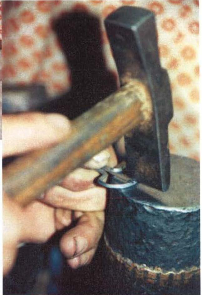
Fig 16. Fixing the tongue in the notch in the frame.
