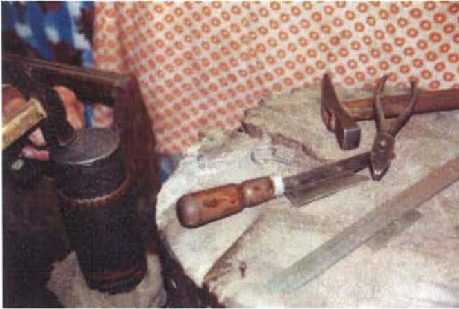
Fig. 14, The tongue requires several operations, from hammering to filing.
